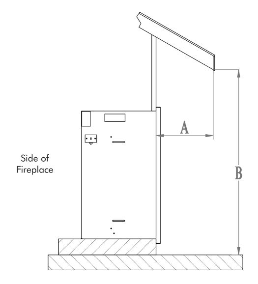
The overhang (A) must extend at least 1/2 the roof-line height (B). Height is measured from the base of the fireplace.
