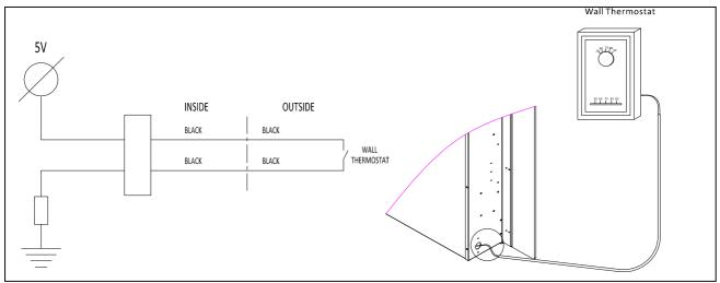
NOTE: The wall thermostat will be functioning when the heater is on the TEMP. setting.
