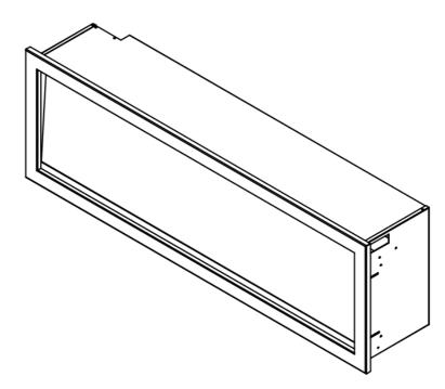
5. Put the fireplace into the wall opening and fix it to the wall by screwing 2 screws each side.
